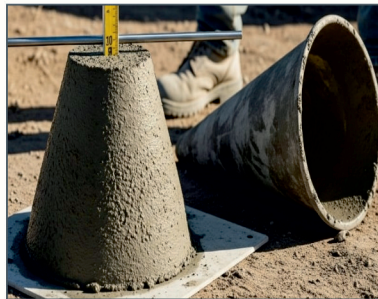
CONCRETE WORKABILITY TEST BY SLUMP CONE METHOD
